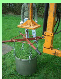
Fig. 1: TME-soil cores are taken with minimal disturbance
